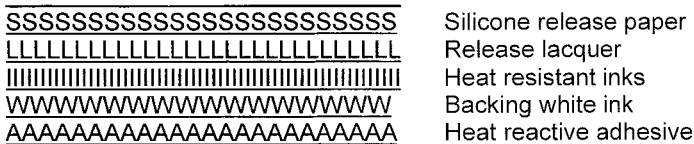
Figure 7.9 A typical heat transfer label structure.
