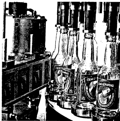
Figure 8.17 Labelling machine applying Avery-Dennison's patented 'CLEAR ADvantage' thermal transfer labels. On the left can be seen the continuous web carrying the label graphics in the form of specially-formulated inks, which are transferred to the glass bottles as the result of a combination of heat and pressure.
