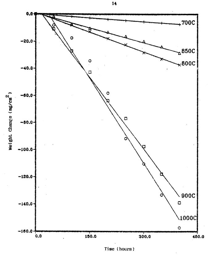
Figure 7. Weight change of alloy 188 with the experimental time.
