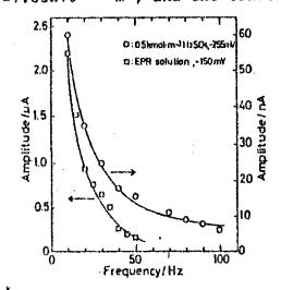
Rig.3 Effect of modulation frequency on laser enhanced current.
