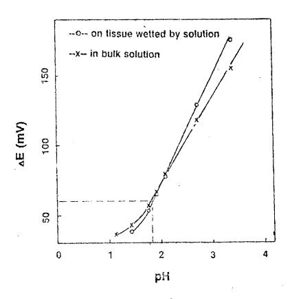
Fig. 2 The characteristic  $\triangle E \sim pH$  curves of  $Sb/Sb_zO_3$  and Ag/AgCl microelectrode couple.
