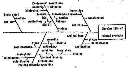
Fig. 1 Cause and Effect diagram of service life of plated products.
