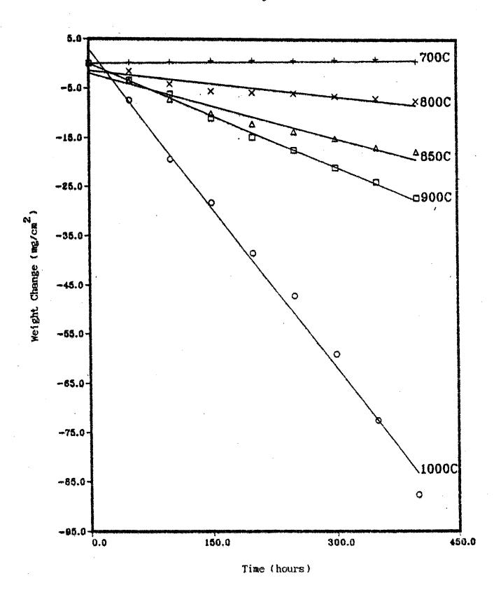
Figure 2. Weight change of alloy 800H with the experimental time.
