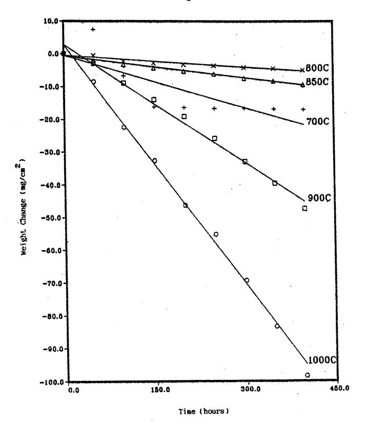
Figure 1. Weight change of alloy 310 with the experimental time.
