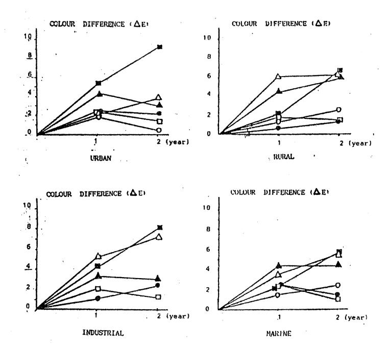
Fig 3.4 Colour difference ( $\triangle E$ ) of specimens at different environments
