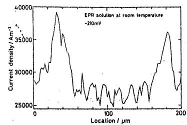
Fig.9 Line profile of laser enhanced current for sensitized Type304 stainless steel kept at -210 mV in the EPR solution, giving the grain boundary image.
