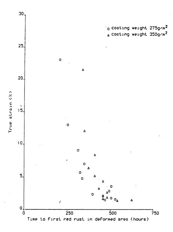
Figure 1: Results of salt spray tests on deformed minimised sheet
