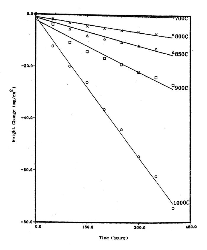
Figure 3. Weight change of alloy 556 with the experimental time.
