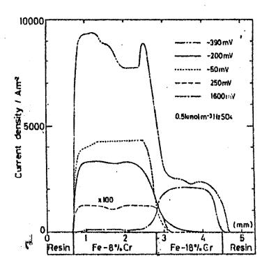
Fig.3 Line profile for the current imaging across the boundary between Fe-8Cr and Fe-18Cr alloys kept at various applied potentials.
