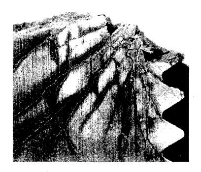
Figure 18. Longitudinal section through the stud-bolt-B showing of branched cracks initiated from one of the thread root (6 X, Kalling's etched).
