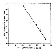
Figure 1. The Effect of Tin Concentration on Electrolyte Nacrothrouing Power
