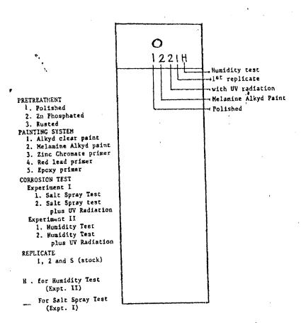
Figure 1. Coding System of Specimens
