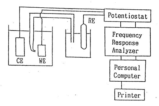
Fig. 2 Block diagram of electrochemical impedance measurement.
