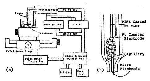
Fig.8 Schematic drawings of (a)the scanning micro impedance probe system and (b)the micro probe.
