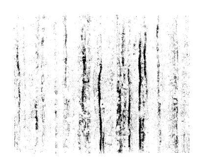
Figure 12. Microstructure of backing plate consists of austenite with elongated carbides (200%, Kalling's etched).
