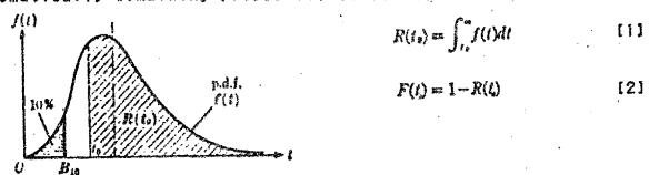
Fig. 2. Failure distribution disgram
