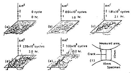
Fig.4 Changes in the distribution of the current density with time during the corrosion fatigue test for high strength steel in synthetic sea water.
