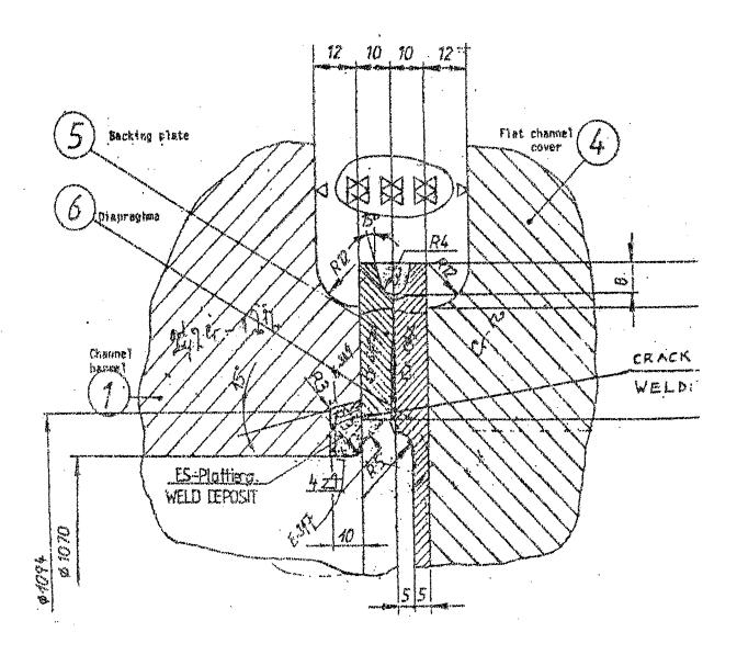
Figure 2. Sample section was taken from backing plate and disphrage for laboratory examination.
