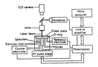
Fig.1 Schematic illustration of SLEEM
