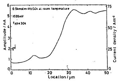
Fig.2 Line profile of the laser enhanced current image scanned across the boundary between resin and Type304 stainless steel polarized at 1020 mV in 0.5 kmol/m H<sub>2</sub>SO<sub>4</sub> at room temperature.
