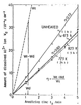
Fig. 4. Time variation in the amount of dissolved  $A\Gamma^{(r)}$  ions,  $W_d$ , during anodizing, for heated and unheated specimens. Conditions of heating and anodizing are as in Fig. 3.
