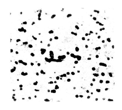
Figure 22. Microstructure of stud-bolt consists of austenite with spheroidize carbides disperse throughout of microstructures (500X, Kalling's etched).
