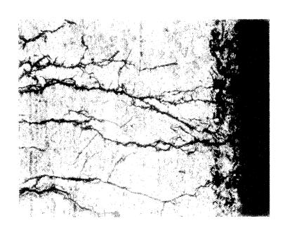
Figure 10. The end of branched cracks lead to the outer surface of diaphragm which it was revealed some pittings corrosion (100%, Kalling's etched).
