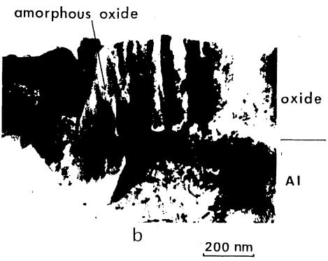
Fig. 8. Electron micrographs of a) the stripped film and b) cross section, obtained from the 5-min-anodized specimens with heat treatment at 823 K for 3 hr. Anodizing conditions are as in Fig. 3.
