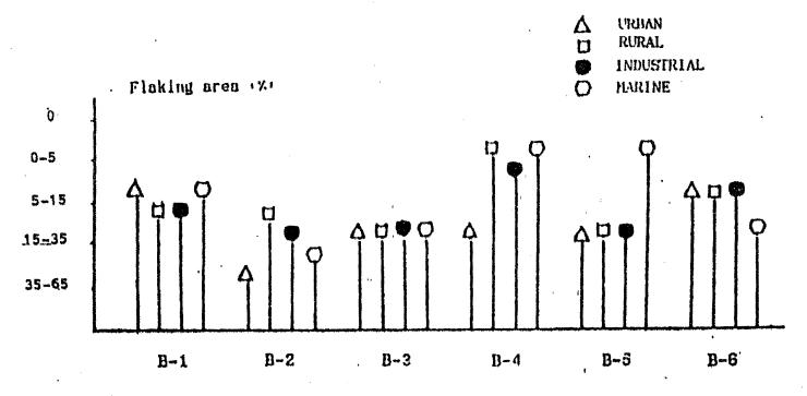
Fig 3.7 Adhension of specimens after 2 years exposure
