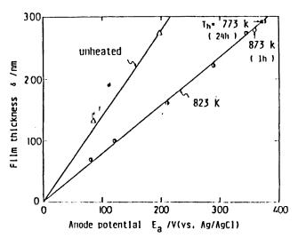
Fig. 7. Relationship between anodic oxide film thickness,  $\delta$ , and anode potential,  $E_a$ , obtained from heated and unheated specimens. Anodizing conditions are as in Fig. 3.
