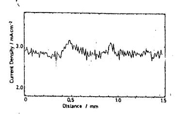
Fig.7 Current distribution on sensitized SUS304 in 0.5M H<sub>2</sub>SO<sub>4</sub> + 0.01M KSCN, showing intergranular corosion current.
