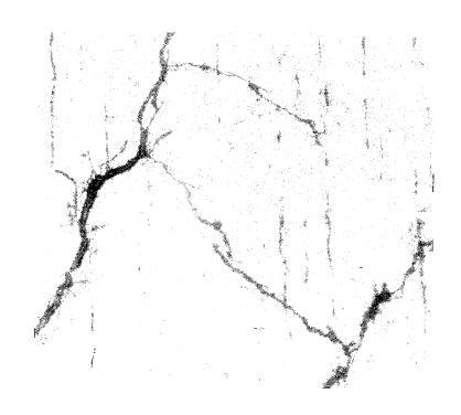
Figure 20. Branched cracks as characteristic of SCC was propagated transgranular (200X, Kalling's etched).
