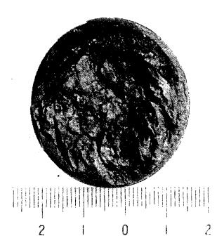
Figure 14. Fracture surfaces of stud-bolt-B revealed brittle, jagged and coated with corrosion deposit (2 X).
