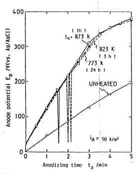
Fig. 3. Time variation in the anode potential,  $E_a$ , during anodizing from heated specimens (at 773 K for 24 hr, 823 K for 3 hr, and 873 K for 1 hr) and unheated specimens. Anodizing was carried out at a constant e.d. of 50 A/dm² in 0.5 mol/dm³ H<sub>2</sub>BO<sub>3</sub>/0.05 mol/dm³ Na<sub>3</sub>B<sub>4</sub>O<sub>3</sub> solution at 353 K.
