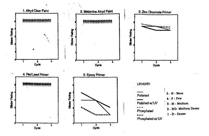
Figure 3a. Blister Rating of Specimens Subjected to Salt Spray Test (Experiment I)
