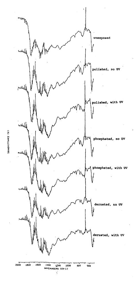
Figure 7. FTIR Spectra of Red Lead Primer Coated Specimens After 7th cycle Humidity Test
