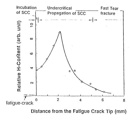
Fig. 4 Hydrogen distribution on the SCC fracture surface of a Ti-5Al-2.5Sn sample in nearly neutral 3.5%wt NaCl solution determined by SIMS.
