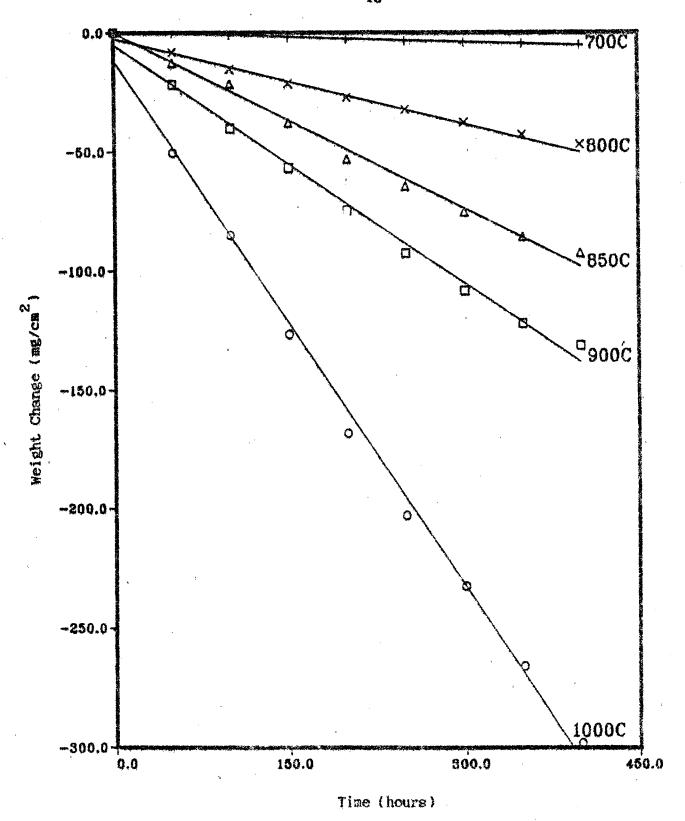
Figure 6. Weight change of alloy C-276 with the experimental time.
