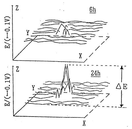
Fig. 8 SVET maps of steel plate coated by VC in 100ppm NaCl solution at room temperature without chemical conversion treatment.
