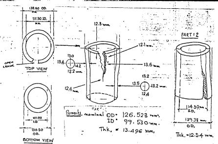
Fig.3 Sketch of the rupturing reformer C-2.
