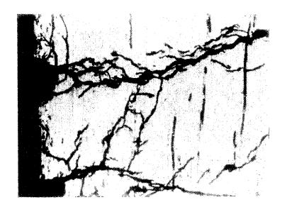
Figure 9. Branched cracks with transgranullar propagation as a characteristic appearance of SCC starting from inner surface of diaphragm (left side), 100 X magnification, Kalling's etched.
