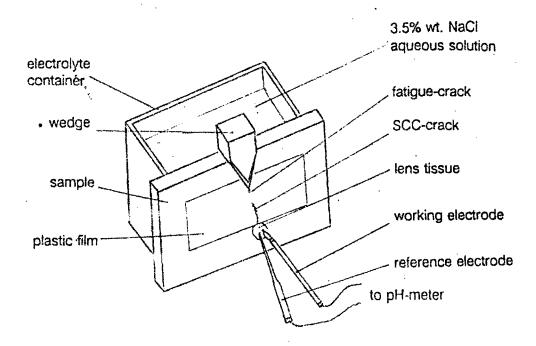
Fig. 1 Schematic diagram of the experimental set-up for the measurement of pH value of the crack tip electrolyte during SCC of titanium alloys.
