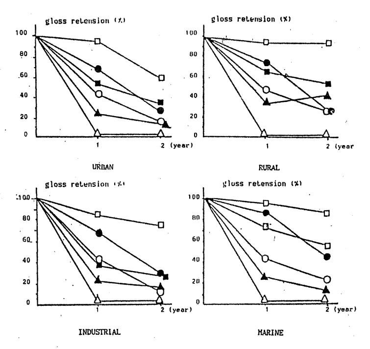
Fig 3.6 gloss retension of specimens at different environments
