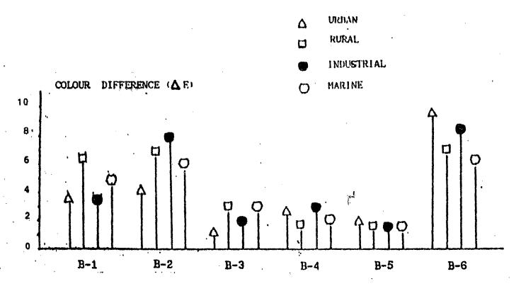
Fig 3.3 Colour difference ( $\Delta E$ ) of specimens after 2 years exposure
