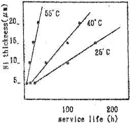
Fig. 8 MI thickness vs. service life
