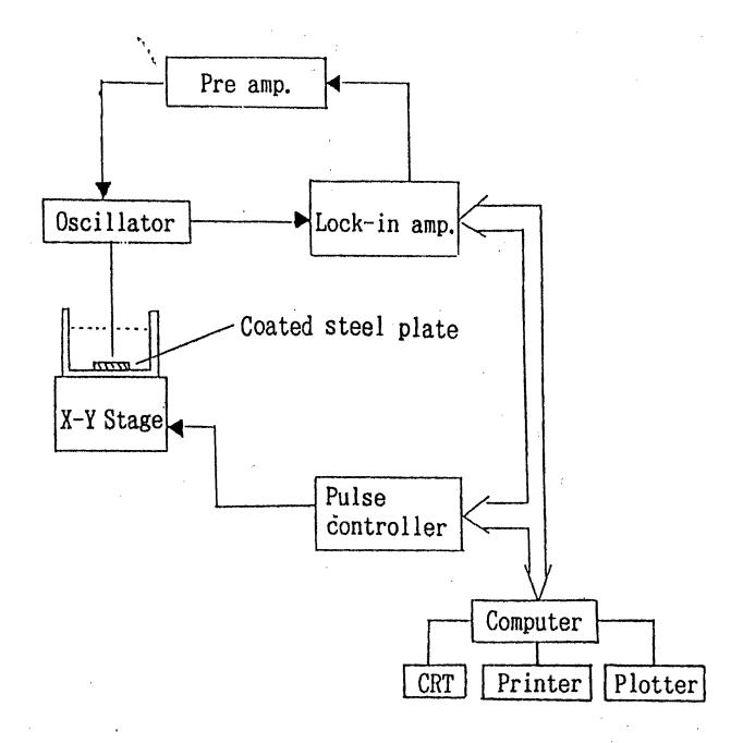
Fig. 3 Block diagram of scanning vibrating electrode technique.
