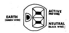
One power contact (the active wire) delivers 220 volts with respect to earth while the other (the neutral wire) is at earth potential. Unfortunately, the convention as to which wire is active is seldom observed in practice and it is essential to treat both power wires as dangerous. When connecting equipment to the power line or operating equipment with which you are unfamiliar, you should observe the following precautions:
