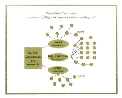
In case the amount of water used by farmers is considerable and the volume of water in Huai Hin Khao Reservoir (small reservoir) is insufficient, water may be conveyed from Pa Sak Jolasid Dam (big reservoir) to Huai Hin Khao Reservoir (small reservoir), which will help refill the volume of water in the farmers' ponds without their having to face the risk of water scarcity.
