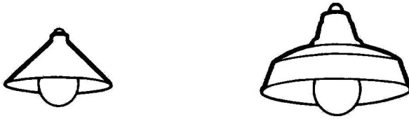
Fig. 52. - Simple conical shades, and reflectors too small for the lamp they carry, give no protection against glare
