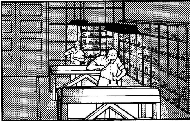
Fig. 54. - Prolonged work in a pool of light in an otherwise badly lit room can cause eye fatigue
