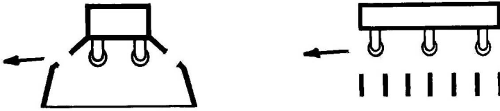
Fig. 45. - Lamps must remain screened throughout the whole of the shielding angle. Troughs with slots cut in the sides, or units with a louvered base but completely open sides are thus unsatisfactory
