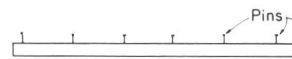
Step 2. Position \frac{3}{16} \times \frac{1}{2} -in. fiberboard divider strips (waxed) with common pins
