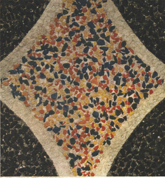
1. Ground surface with ceramic aggregates.
