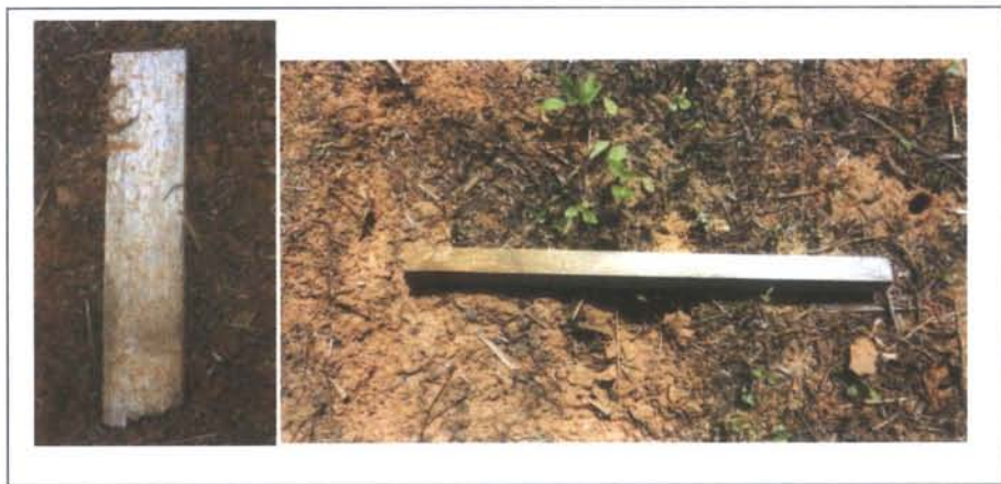
Figure 4. Rejected 0.4x3.8x25.4 cm. and 1.9x1.9x45 cm. Ai sample sizes
