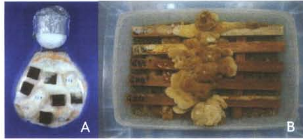
Figure 5. Experimental method (A) Agar block test and (B) Wood stick sandwich method.
