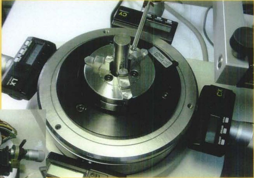
The turntable disassembled. This dish turns "true" within 25 nm (.000001 in) typically.
