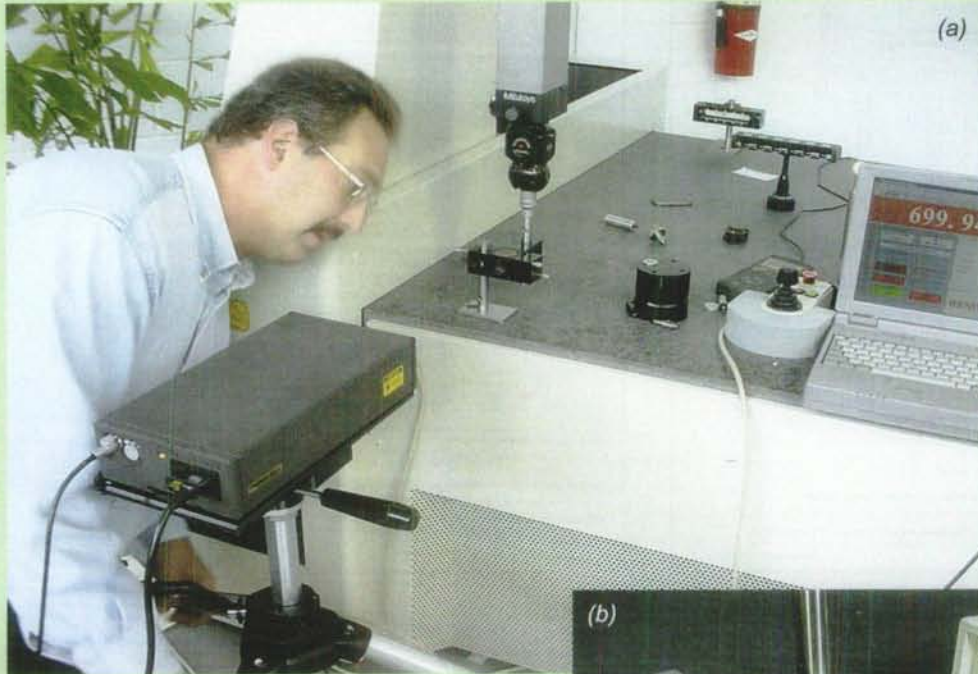
(a) Renishaw's He-Ne laser calibration equipment being used to calibrate a CMM.
