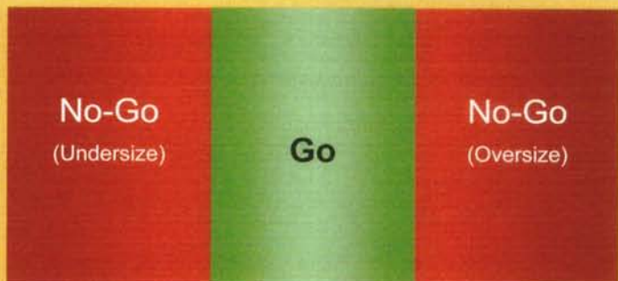
In reality, a production run is separated into three categories by the Go/No-Go method. Oversized shafts are returned for reworking, while the undersized shafts are scrapped.
