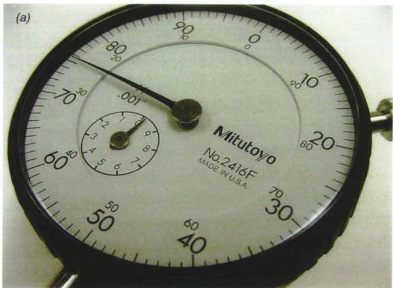
AGD specified Series 2 Dial Indicator
