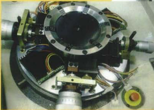
The turntable disassembled. This dish turns "true" within 25 nm (.000001 in) typically.
